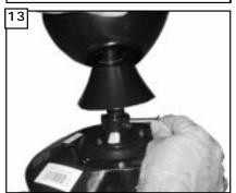
Place downrod into the yoke, align the holes in the yoke with the holes in the downrod and install cross pin.
